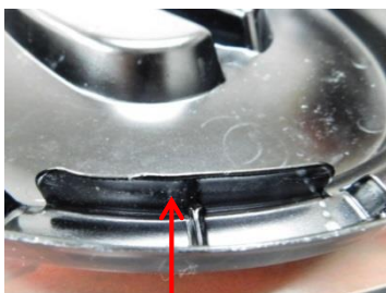
Actuator ridge on Ice Bin lid
