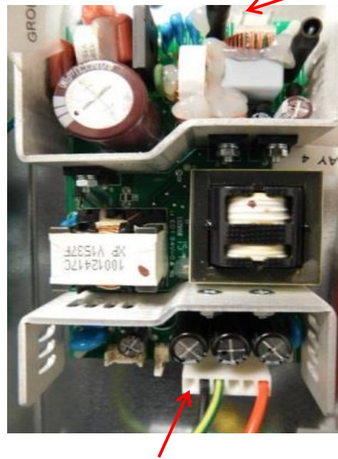
24VDC voltage terminal J2
